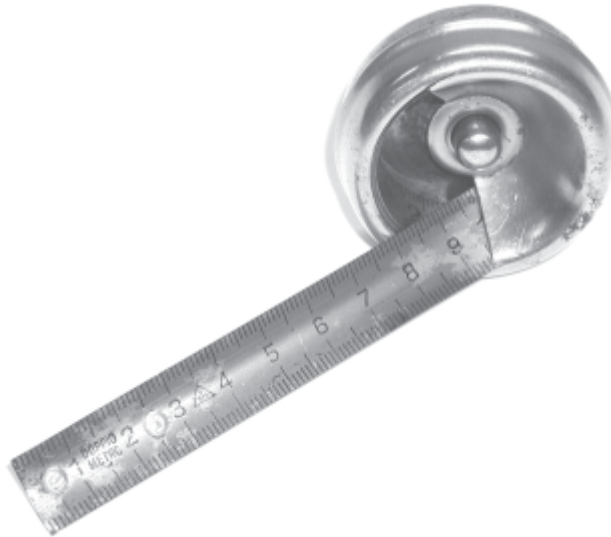
Fig. 1: An early (around 1950) example of a tape measure made from a thin cylindrical steel shell. The structure is monostable: it is only in a stable equilibrium state when it is extended. When coiled, the structure must be held within its housing.
